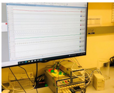
PowerLab 16 channel recorder with accessory (cardiac output kit, bridge amp, ECG kit, pressure transducer kit)
